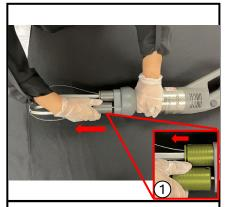
**Step 1: Remove the whisks:** pull down on the whisk ejectors to release whisks as seen on diagram 1
